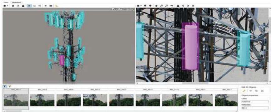
For instance, detectors trained through machine learning can automatically identify objects in photos and defects on a structure, then localize them in the model. It is very useful to automatically classify equipment like pumps or valves in a plant, lighting poles or street furnitures in a city or cracks on a dam or bridge.
