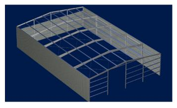
Multiple materials can be used in your RAM Elements models as shown in this warehouse that combines built-up steel rafters and girders, hot-rolled steel columns, cold-formed purlins and girts, plus a perimeter CMU wall.
